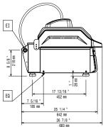
Electrical inlet (power) Electrical Outlet
